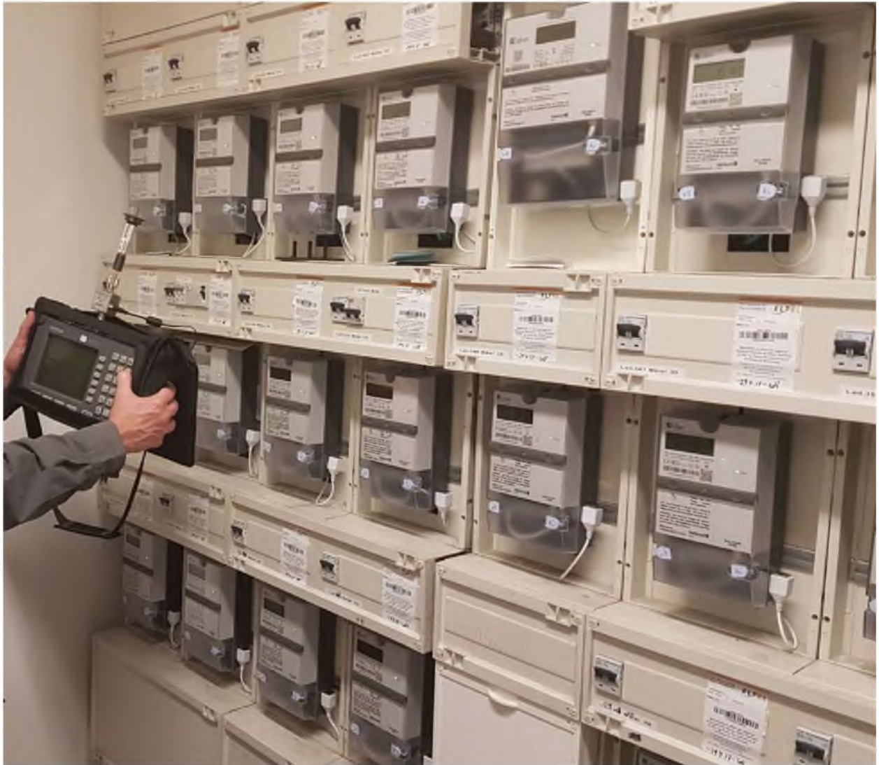
High Frequency EM radiation measurement (HF registration of sources in AMS room 1)
