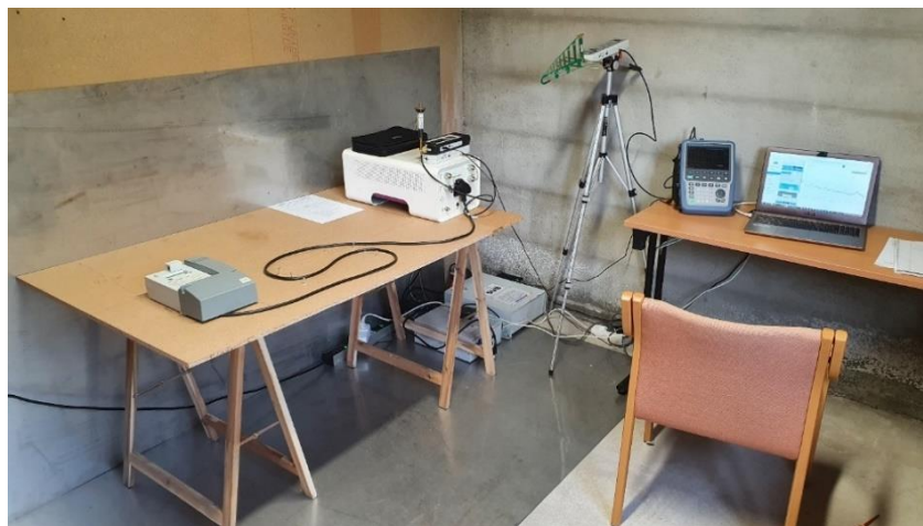
The test setup with EMZER-EMSCOPE to the right and electricity meter to the left on the table.
