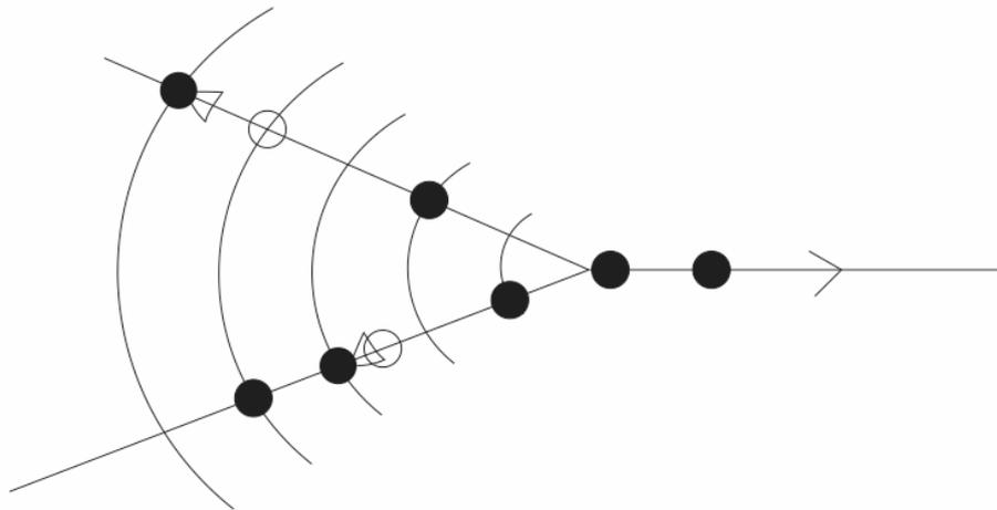
Figure. With point-synchronous control the merge controller will allocate passage times to approaching vehicles so that they pass the merge at safe headways and at nominal speed.
