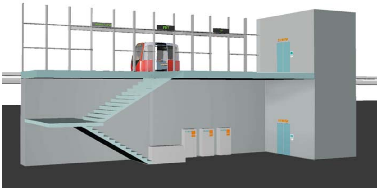
Low capacity station: ticketing, admission control, elevator and stairs. Glass wall with sliding doors towards track
