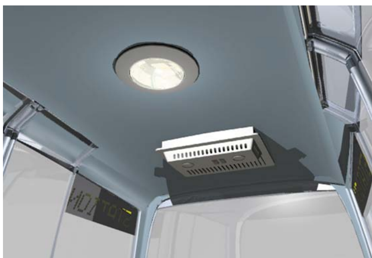
Vehicle interior – with air conditioning system
