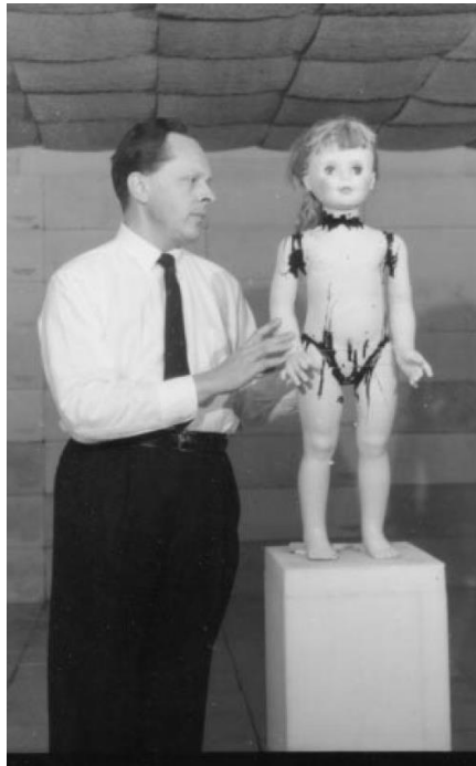
Figure 1 "Schwan with model of human body used for RF dosimetric studies. The model is filled with tissue-equivalent liquids and exposed to RF energy in a microwaveanechoic chamber that Schwan had constructed in his laboratory."(Foster, 2002, p. 20)
