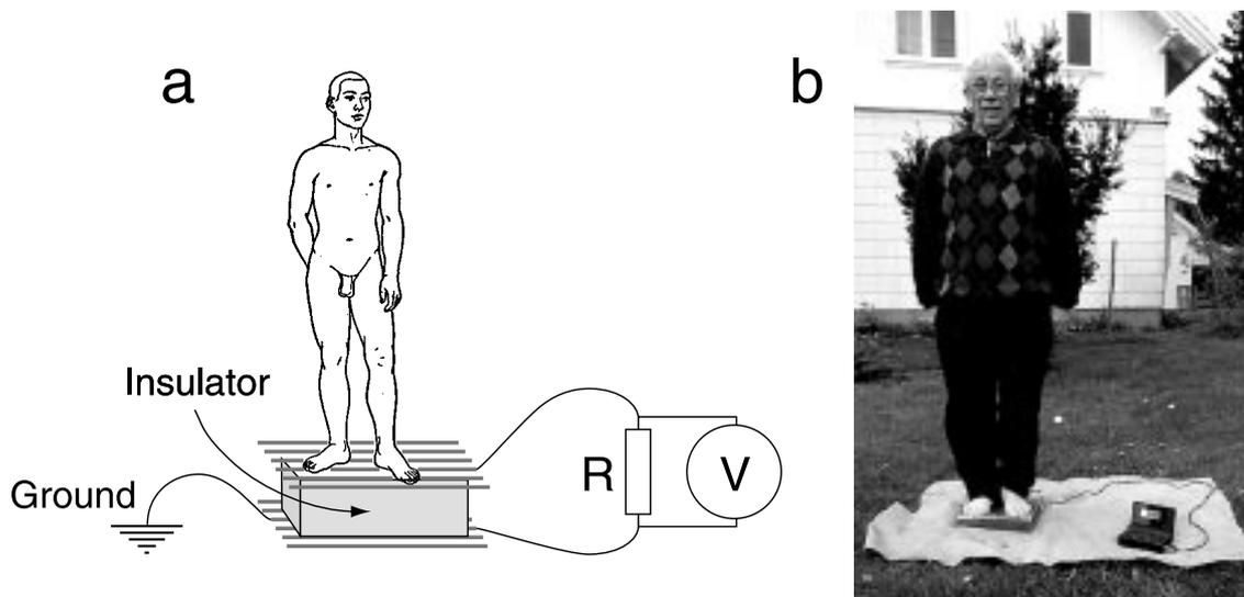
Figure 10-10. Measurement of the alternating current flowing between a human body and ground in an external AC electric field. The principle used in the measurement is given in **a**, and in **b** an actual measurement situation is illustrated.
