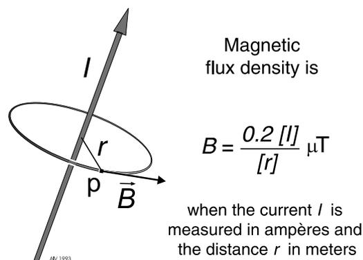
Figure 10-3. Magnetic field at a distance  $r$  from a straight wire carrying an electric current  $I$ .
