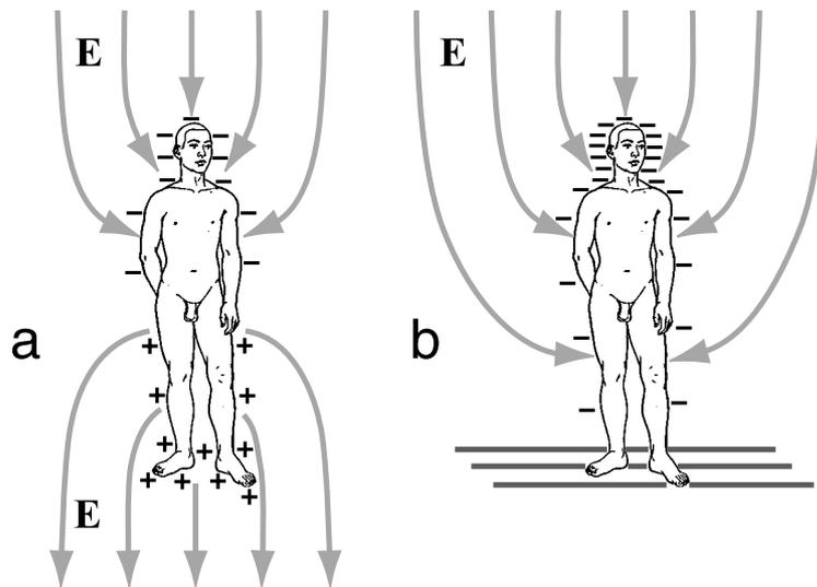
*Figure 10-9. A human body in an external electric field. In **a** the body is insulated from ground, and in **b** the body is grounded through the feet. The charges that accumulate on various parts of the body is for clarity reasons drawn just outside of the body. In reality the charges are located in a thin layer in the skin.*
