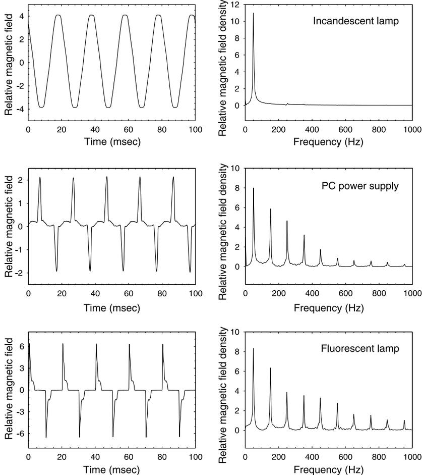
*Figure 10-6. Almost harmonic and clearly non-harmonic time-variations of magnetic fields close to an incandescent, a PC power supply, and a fluorescent lamp, respectively. Frequency analysis shows that the almost harmonic signal contains almost only one frequency, while the non-harmonic signals contains many frequencies.*
