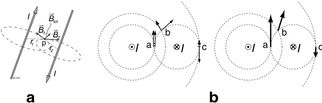
Figure 10-4. Magnetic field from two straight wires both carrying an electric current  $I$ , but in opposite directions. In **a** the wires are drawn in perspective, in **b** the magnetic field is given in a plane perpendicular to the wires. Separate contributions from the two wires (left) and the total field (right) is drawn for three different positions. One can easily see that the magnetic field is stronger between than outside the wires.
